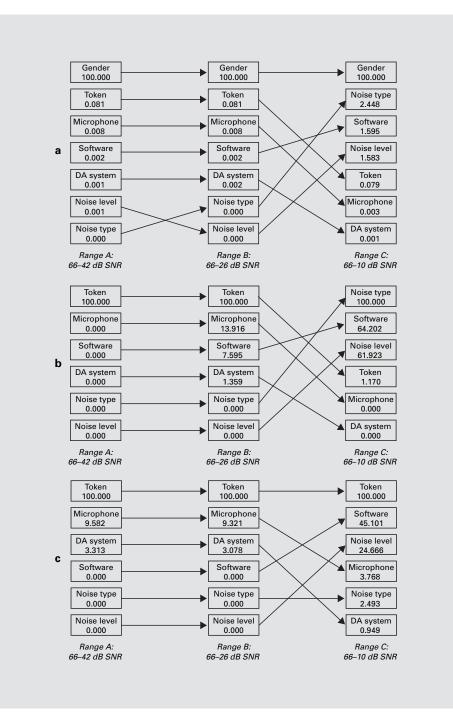
**Fig. 4.** Block diagram of the factor order and specific VIM for  $F_0$  across the three SNR ranges for all (a), female (b), and male (c) participants.
